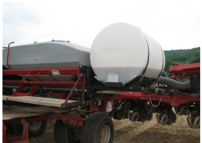
Figure 2. Tank attached to planter for liquid fertilizer application.
