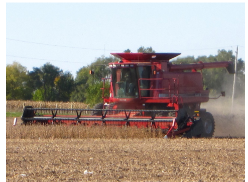
Figure 1. Most mechanical seed loss or seed shattering occurs at the gathering unit, between the header and standing soybean plants.
