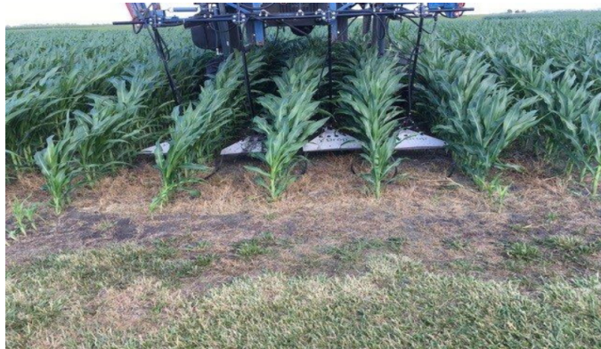
Figure 4. A 360 Y-Drop® applicator can be used to apply N as a sidedress or to corn prior to tasseling.
